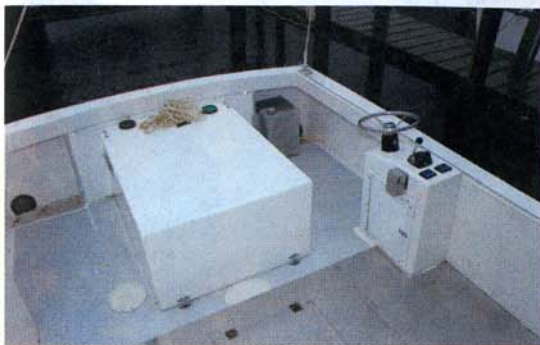
Aluminum plating to protect the fiberglass and plywood deck from shovels stops just before the stern drive's engine box.
